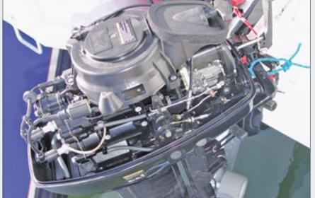
normally, it fired first pull every time and although it occasionally needed a minute or two to settle down. especially if it had been manhandled around the marina and garage, then it would carry a bit more oil in the cylinders and be smokier than we're used to these days. But it is a 2-stroke and that's what 2-strokes do - they can't help themselves because the oil has to be added to the petrol to lubricate the engine's operating system.
